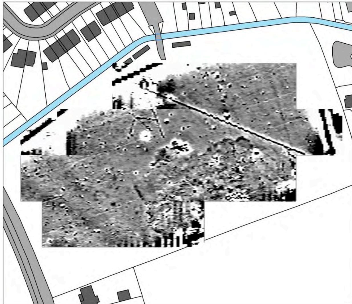
trace) Figure 9. Processed real time gradiometer data (grey
