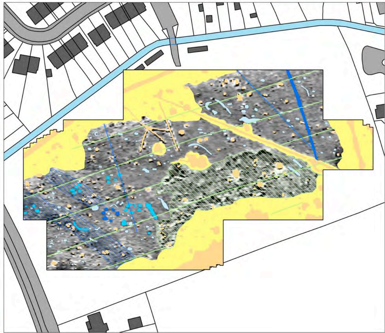
scale) Figure 10. Processed real time gradiometer data and interpretation
